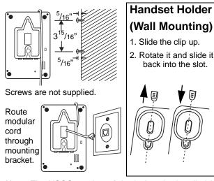
Note: The USOC number of the jack to be installed is RJ11C (RJ11W for a wall jack).
